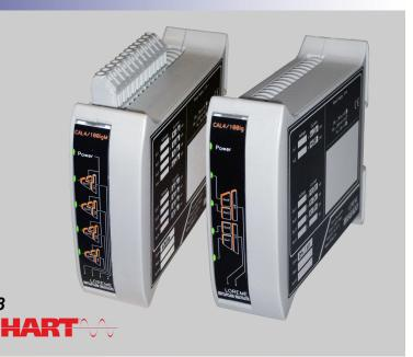
Series of galvanic isolators composed of several independent cells designed for the 0..4..20mA current loop processing. Each input may be wired in active or passive mode, so it is able to measure a current provided by an active transmitter or to supply a 2-wire transmitter and measure the loop current.
